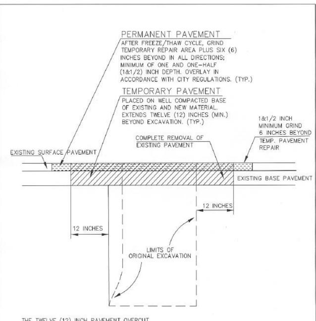
THE TWELVE (12) INCH PAVEMENT OVERCUT MEASUREMENT STARTS AT FURTHEST EDGE OF INTACT NATIVE SOILS. TRENCH WALL DISTURBANCE WILL IMPACT AMOUNT OF PAVEMENT REMOVAL REQUIRED.
