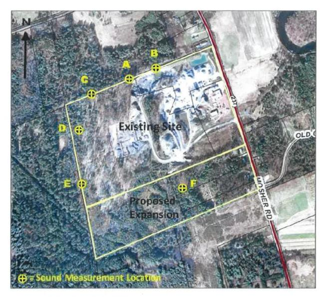
Figure 4-1. Sound Measurement Locations
